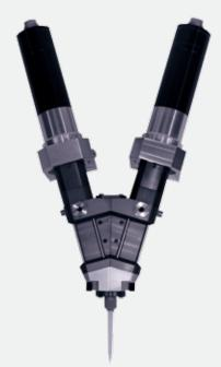
The 2-component ViscoDuo-V 4/4 dispenser is a valveless, static mixing head with dispensers located directly in front of the mixer. The mixing head functions valve-free. The components to be mixed are dosed by volume only and with no dead space into the static mixing tube via the dispensers.
